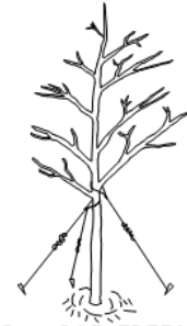
FOR LARGE TREES. SPRINGS IN THE GUY PROVIDE FLEXIBILITY.
