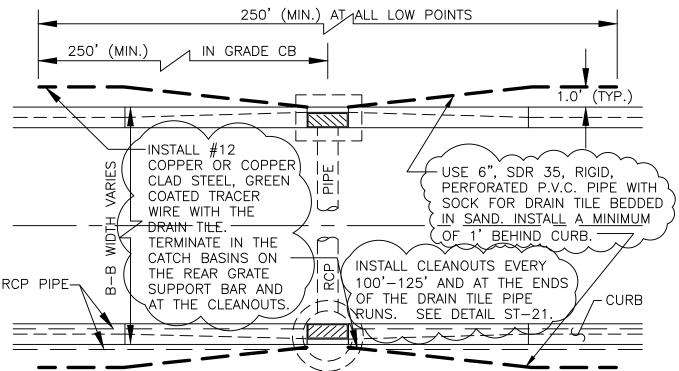
6" RIGID PERFORATED DRAINTILE IS REQUIRED AT ALL LOW POINT CATCH BASINS AND ON THE UPHILL SIDE OF ALL IN-GRADE CATCH BASINS. BENDS MAYBE USED UP TO 22  $\frac{1}{2}$  DEGREES WITH THE RIDGID DRAIN TILE. FLEXIBLE 6" DRAIN TILE CAN BE USED IN CUL-DE-SACS.
